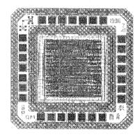
Figure 6. The VLSI Layout of Divider
