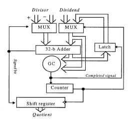
Figure 2. The Architecture of the Divider
